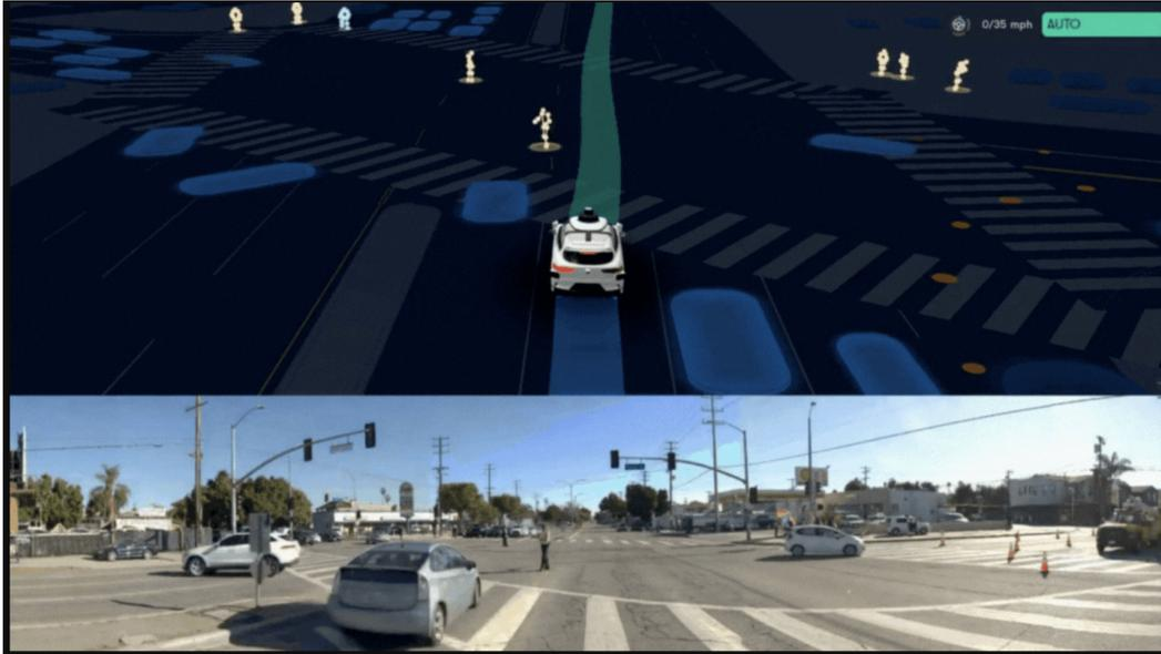
Figure 1.1: [Waymo simulation](#) uses sensors, including cameras and LiDARs, to reconstruct the environment. This below figure shows the view captured by the camera while the above figure depicts the reconstructed environment, with detected humans and vehicles denoted in blue, the crosswalk in white, and the planned trajectory shown in green.
