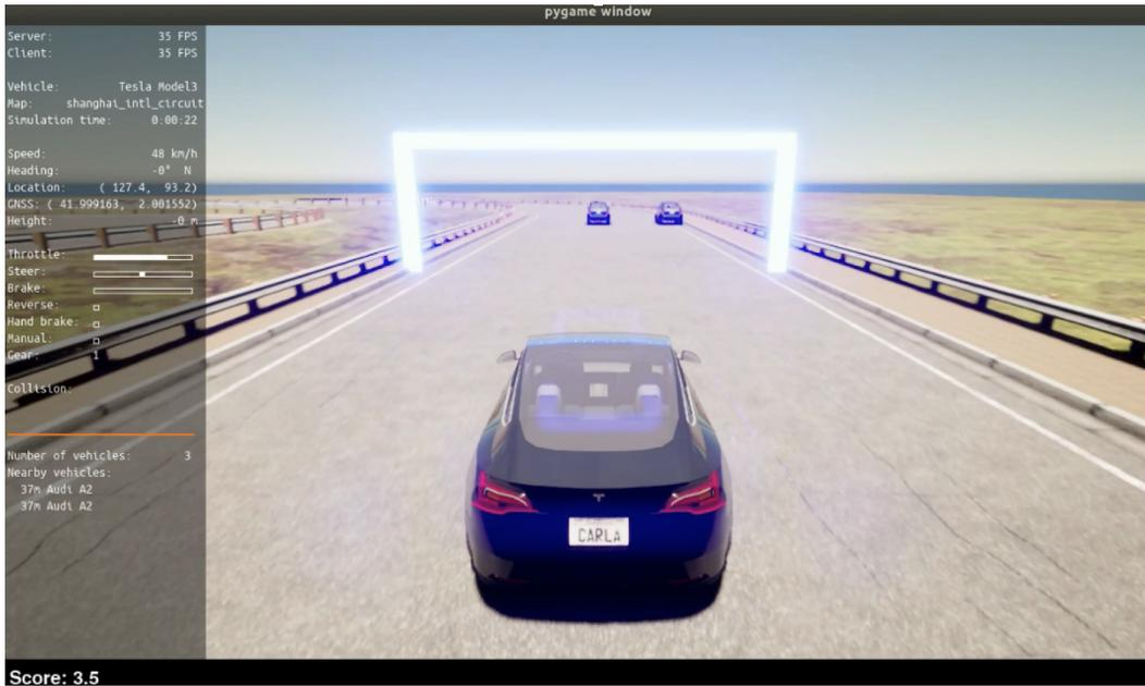
Figure 2.4: An example of the GRAIC Scenario. The blue box in front of the ego vehicle is the waypoint it requires to reach. The two vehicles ahead are the dynamic obstacles that the ego vehicle is expected to avoid. One controller design choice is to change to the left lane and overtake the obstacles using the inside lane of the left turn ahead of the ego vehicle.
