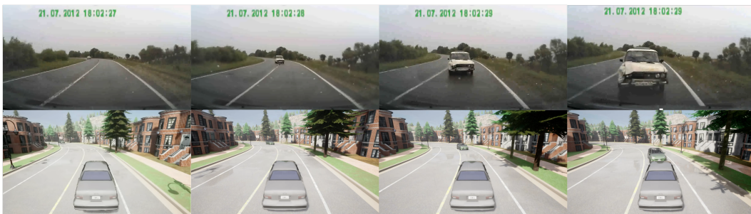
Figure 5: Opposite Vehicle Invading Lane Scenario: in the original dash camera video (top row), the vehicle on the opposite lane gradually swifs to ego's lane probably due to loss of focus. In the generated scenario (bottom row) produced by our framework, the vehicle on the opposite lane exhibited a similar lane change behavior to switch to our lane and caused collision.
