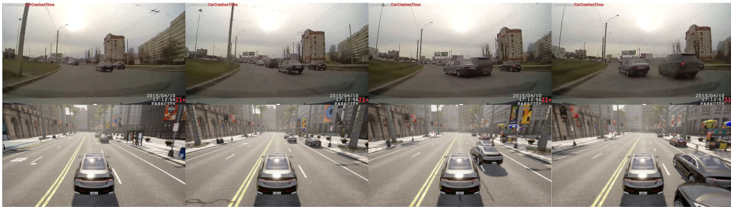
Figure 8: Vehicle Cutting In with Stopped Object Scenario : in the original dash camera video (top row), the vehicle on the right perform an emergency brake and tried lane change to the left due to a front parked vehicle. In the generated scenario (bottom row) produced by our framework, the vehicle on the right exhibited a similar lane change behavior to the left to avoid the stopped vehicle and cause a collision.
