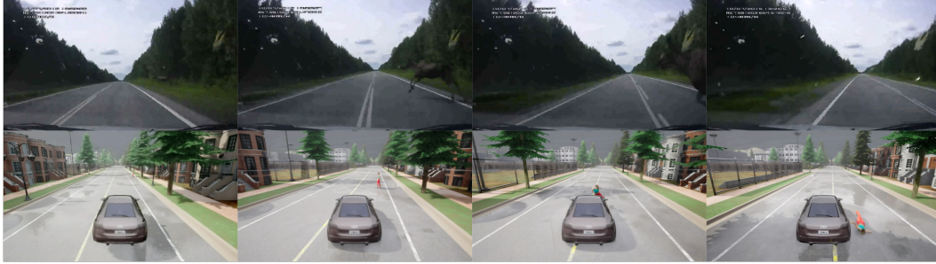
Figure 7: Animal Crossing Scenario : in the original dash camera video (top row), an animal attempted to cross the road, prompting the ego vehicle to perform an emergency lane change to the left. In the generated scenario (bottom row) produced by our framework, the ego vehicle exhibited a similar lane change behavior to the left to avoid a jaywalking pedestrian (since CARLA does not have an animal model, the animal is replaced by a pedestrian).
