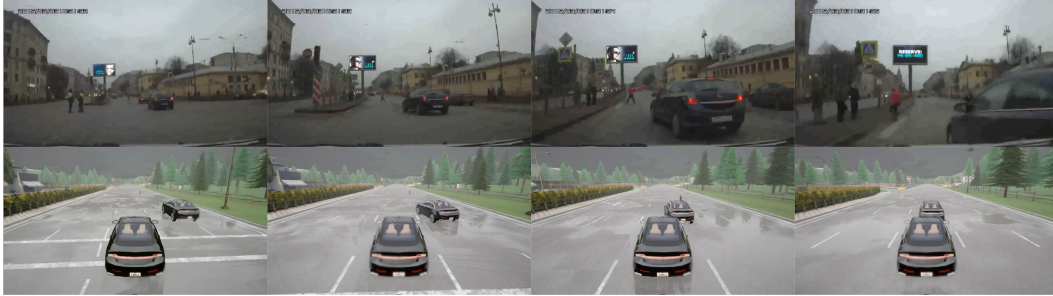
Figure 4: Vehicle Cutting In with Pedestrian Crossing Scenario: in the original dash camera video (top row), the vehicle on the right performs an emergency lane change to the left due to a jaywalking pedestrian in red. In the generated scenario (bottom row) produced by our framework, the vehicle on the right exhibited a similar lane change behavior to the left to avoid a jaywalking pedestrian.
