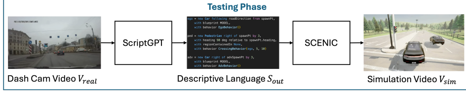
Figure 2: After prompt engineering, the dash cam video is fed into ScriptGPT , which synthesizes descriptive language in the SCENIC format. This SCENIC script can then be executed in CARLA to generate a corresponding testing scenario in simulation.
